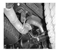
INSTALL OVERAXLE TAILPIPE #C INTO THE REAR OF THE MUFFLER. SLIP THE HANGER INTO THE FACTORY RUBBER GROMMET. USE CLAMP #H AT THE REAR OF THE MUFFLER, BUT DO NOT TIGHTEN.
