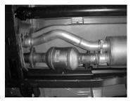
MUFFLER MUST BE WELDED ON THE PASSENGER SIDE INLET AND CLAMPED ON THE DRIVER SIDE INLET WITH CLAMP #G. DO NOT WELD UNTIL KIT IS COMPLETELY INSTALLED.
