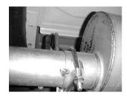
Install muffler onto head pipe 1-1/2" to 2" with the louvers facing towards the converter. Use a jack stand to support the muffler. Use clamp #G to secure the muffler to the head pipe. Insert hanger into rubber grommet. Do not tighten. Muffler inlet is looking into the louvers.
