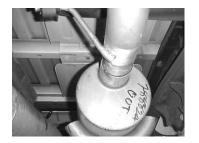
Install the tailpipe # C into the muffler at least 1-1/2" to 2". Secure pipe to the muffler using clamp # E. Do not tighten. Insert welded hanger into rubber grommet.
