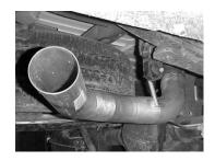
Install exit pipe #D onto the tailpipe.
