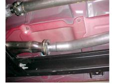
BOLT HEADPIPE #A TO THE STOCK FLANGE RE-USING THE FACTORY NUTS & BOLTS. INSERT WELDED HANGER INTO RUBBER GROMMET.
