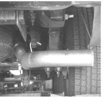
INSTALL EXIT PIPE #D INTO OVERAXLE TAILPIPE USING CLAMP# E. ROTATE EXIT PIPE UNTIL IT IS AT THE CORRECT ANGLE FOR YOUR TRUCK. INSERT WELDED HANGER INTO RUBBER GROMMET.
