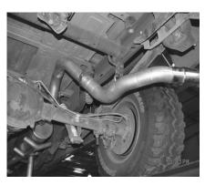
INSTALL OVERAXLE TAILPIPE #C TO THE OUTLET OF THE MUFFLER USING CLAMP #E. INSERT WELDED HANGER INTO RUBBER GROMMET.
