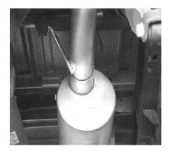
NEXT CONNECT THE MUFFLER TO THE HEADPIPE USING CLAMP #E. USE JACKSTANDS TO SUPPORT THE MUFFLER. THE OUTLET OF THE MUFFLER WILL BE AT APPROXIMATELY 11 O'CLOCK. THE MUFFLER INLET IS LOOKING INTO THE LOUVERS.
