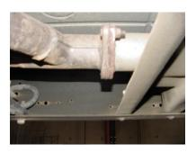
TO REMOVE STOCK EXHAUST UN-BOLT THE FACTORY FLANGE LOCATED IN FRONT OF THE MUFFLER. DO NOT THROW AWAY THE STOCK BOLTS AND NUTS. YOU WILL RE-USE THEM.
