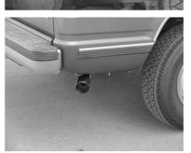
INSTALL STAINLESS TIP. USE ANY ALUMINUM OR STAINLESS CLEANER TO POLISH YOUR TIP. TIGHTEN ALL NUTS, BOLTS & CLAMPS.
