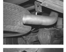
INSTALL TURNOUT #D PIPE ONTO TAILPIPE.
