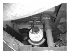
INSTALL MUFFLER ONTO HEADPIPES NO MORE THAN 1 ½" TO 2" USING CLAMPS #G. USE A JACKSTAND TO SUPPORT MUFFLER.
