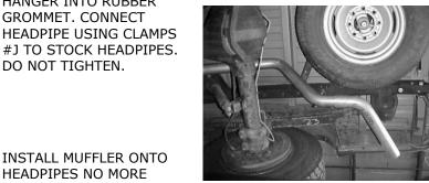
INSERT TURNOUT PIPE #E ONTO TAILPIPE AND ROTATE FOR YOUR DESIRED LOOK. USE CLAMP #H TO CONNECT TAILPIPE AND TURNOUT PIPE TOGETHER. DO NOT TIGHTEN.
