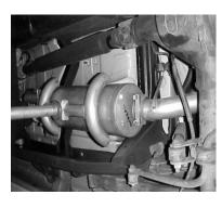
SLIDE MUFFLER WITH DUAL INLET ONTO HEADPIPE AT LEAST 1-1/2" TO 2".
