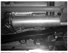
Install muffler #A onto factory headpipe with the flange end of the muffler using gasket #E and using bolt kit #F, Make sure the outlet of the muffler is at the 4 o'clock position. Do not tighten.
