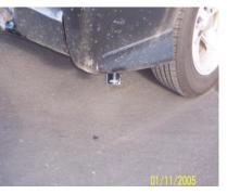
Install stainless steel tip. Clamp down. To clean stainless steel tip, use a scotch brite pad and any stainless steel or aluminum cleaner. When you have everything in place, firmly tighten all bolts and clamps.
