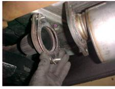
Lay out the GIBSON EXHAUST SYSTEM on the floor so it looks like the drawing and match the part numbers with the parts list. (Note: Drawing is not exact except for placement of parts only!) Raise vehicle and support with stands. Unbolt stock exhaust in front of your stock muffler. Leave all rubber mounting grommets in place. Use WD-40 to aid in removal of hangers.
