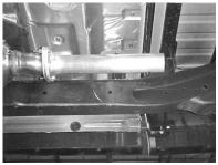
REMOVE STOCK EXHAUST BY UNBOLTING IT FROM THE 2 BOLT FLANGE JUST IN FRONT OF THE CONVERTER. DO NOT REMOVE STOCK STUDS. LEAVE ALL RUBBER GROMMETS IN THE STOCK POSITION. USE WD-40 TO AID YOU IN REMOVING THE RUBBER GROMMETS FROM THE STOCK HANGERS. FOR EASIER REMOVAL CUT THE TAILPIPE JUST BEHIND THE MUFFLER.
