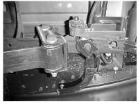
REMOVE FACTORY REAR TAILPIPE EXHAUST HANGER FROM FRAME.
