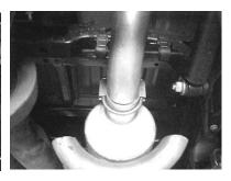
INSTALL REAR MUFFLER HANGER #H TO MUFFLER OUTLET AND INSERT WELDED HANGERS INTO RUBBER GROMMETS AND CLAMP.
