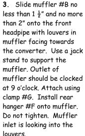
MAKE SURE YOU HAVE A 1" CLEARANCE ON ALL PIPES FROM RUBBER BRAKE LINES, FUEL LINES, SHOCK BOOTS, TIRES, ETC ...
