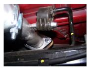
3. Install headpipe #A onto your existing stock flange using bolt kit #F to secure flange. DO NOT TIGHTEN. Insert welded hanger into rubber grommet.
