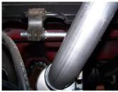
5. Install tailpipe #C into muffler approximately 1½-2". Secure tailpipe with clamp #E. DO NOT TIGHTEN. Insert welded hanger into rubber grommet.
