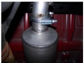
GIBSON EXHAUST systems are designed on a factory stock vehicle. Any aftermarket products installed could increase the sound levels of the exhaust. Make sure there is a 1" clearance from ALL rubber brake lines, shock boots, lines, tires, etc. to prevent heat related damage or fire.
