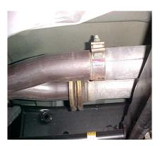
Lay out the exhaust on the floor so it looks like the drawing and compare parts with manual. To remove the stock exhaust remove it from the stock flange & slip joint located in front of the muffler, then cut off your tailpipe just behind the muffler. Use WD-40 to aid in removal of hangers from grommets leave grommet on vehicle.
