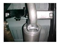
Install rear muffler hanger #F onto outlet of muffler. And clamp down to tailpipe. Insert hanger into rubber grommet. Do not tighten.
