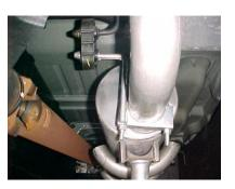
Install muffler #C onto head pipes 1-1/2" to 2"with the louvers facing towards the converter. Use a jack stand to support the muffler. Use clamps #G to secure the muffler to the head pipes. Do not tighten. Outlet of muffler should be at 6 o'clock.
