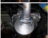
3. INSTALL MUFFLER # B ONTO HEAD PIPE # A 1½"-2" WITH THE LOUVERS FACING TOWARDS THE CONVERTER. USE A JACK STAND TO SUPPORT THE MUFFLER. USE CLAMP # E. TO SECURE THE MUFFLER TO THE HEAD PIPE. DO NOT TIGHTEN. MUFFLER INLET IS LOOKING INTO THE LOUVERS. OUTLET OF MUFFLER WILL BE AT THE 1 O'CLOCK POSTION.
