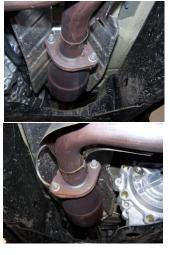
1. LAY OUT THE GIBSON EXHAUST ON THE FLOOR AND COMPARE PART #'S TO THE DRAWING. TO REMOVE THE STOCK EXHAUST REMOVE IT FROM THE 2 BOLT FLANGES, LOCATED IN FRONT OF YOUR FACTORY MUFFLER. NEXT, UNBOLT FACTORY Y-PIPE FROM THE 2 2-BOLT FLANGES.
