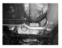
INSTALL Y-PIPE # A ONTO YOUR EXISTING STOCK FLANGES. INSERT HANGER INTO RUBBER GROMMET. USE YOUR FACTORY HARDWARE TO SECURE. DO NOT TIGHTEN.
