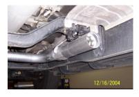
NEXT, INSTALL RESONATOR # B 1 1/2"-2" ONTO Y-PIPE USE CLAMP **# G TO SECURE PIPES** TOGETHER, DO NOT TIGHTEN.
