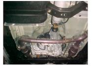
NEXT, UN-BOLT YOUR EXHAUST FROM THE 2-BOLT FLANGES LOCATED JUST BEHIND YOUR FACTORY CATALYTIC CONVERTERS, DO NOT DISGUARD YOUR FACTORY GASKETS AND HARDWARE YOU WILL RE-USE IT. ALSO
