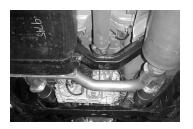
INSTALL Y-PIPE #A ONTO YOUR EXISTING STOCK FLANGES. INSERT HANGER INTO RUBBER GROMMET. USE YOUR FACTORY HARDWARE TO SECURE. DO NOT TIGHTEN.
