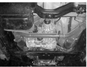
LAY OUT THE GIBSON EXHAUST ON THE FLOOR AND COMPARE PART #'S TO THE DRAWING. TO REMOVE THE STOCK EXHAUST REMOVE IT FROM THE 2 BOLT FLANGES, LOCATED IN FRONT OF YOUR FACTORY MUFFLER. NEXT, CUT OFF YOUR STOCK TAILPIPE BEHIND YOUR MUFFLER. DO NOT DISGARD YOUR FACTORY HARDWARE, YOU WILL RE-USE IT.
