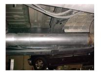
NEXT, INSTALL RESONATOR # B 1 ½"-2" ONTO Y-PIPE USE CLAMP # G TO SECURE PIPES TOGETHER, DO NOT TIGHTEN.
