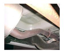
TO REMOVE YOUR STOCK EXHAUST REMOVE IT FROM THE CLAMP LOCATED JUST IN FRONT OF YOUR STOCK MUFFLER.
