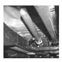
INSTALL THE HEADPIPE RE-USING THE FACTORY GASKET AND BOLTS. APPLY A SMALL AMOUNT OF HI-TEMP GASKET SEALER ONTO THE GASKET TO ENSURE A LEAK FREE CONNECTION. DO NOT TIGHTEN.
