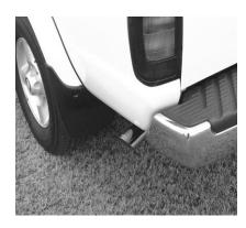
NEXT INSTALL YOUR STAINLESS STEEL TIP TO YOUR DESIRED LOOK. USE A STAINLESS OR ALUMINUM CLEANER TO POLISH TIP. NOW TIGHTEN ALL HANGERS AND CLAMPS STARTING FROM THE FRONT WORKING BACK.
