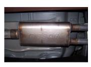
4. Slide muffler #B onto headpipe 1.5-2". Use a jack stand to support the muffler. Use clamp #F to secure the muffler to the headpipe. Do not tighten.
