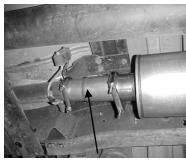
INSTALL HEADPIPE # A USING CLAMP #F AND ATTACH TO THE STOCK EXTENSION PIPE.
