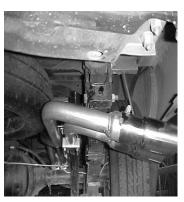
ROLL TAILPIPES UNTIL YOU HAVE IT AT THE CORRECT ANGLE FOR YOUR VEHICLE. NOW FIRMLY TIGHTEN ALL BOLTS, CLAMPS, AND FLANGES.
