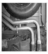
REMOVE STOCK REAR HANGER FROM THE FRAME ON PASSENGER SIDE. INSTALL HANGER #H THROUGH THE LARGE HOLE 19" FROM THE REAR OF THE FRAME. USE NUT AND BOLT SUPPLIED WITH HANGER. INSTALL OVERAXLE TAILPIPES #C, #D. USE CLAMPS #F AT THE OUTLET OF THE MUFFLER TO ATTACH. INSERT WELDED HANGERS INTO RUBBER GROMMET, DO NOT TIGHTEN.
