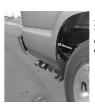
INSTALL STAINLESS STEEL TIPS. USE ANY ALUMINUM OR STAINLESS STEEL CLEANER TO POLISH TIPS.
