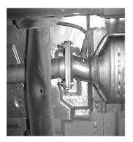
UNBOLT THE STOCK EXHAUST AT THE FLANGE BEHIND THE CONVERTER. FOR EASIER REMOVAL OF EXHAUST USE WD-40. BOLT HEADPIPE #A TO STOCK FLANGE USING BOLT KIT #K AND GASKET #I AND INSERT WELDED HANGER INTO RUBBER GROMMET. USE A JACK STAND TO SUPPORT CONVERTER TO PREVENT IT FROM DROPPING.
