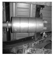
CONNECT MUFFLER #B TO HEADPIPE USING CLAMP #G. INLET IS FACING THE MOTOR. USE A JACK STAND TO SUPPORT MUFFLED
