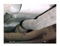
Lay out the exhaust on the floor so it looks like the drawing and compare parts with manual. To remove the stock exhaust un-bolt it from the flange located in front of the muffler. You will re-use your stock hardware. Leave all rubber grommets in place. Use WD-40 to aid in removal of exhaust and the hangers. Cut your stock tailpipe off just behind the muffler.
