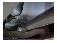
Install head pipe # A onto you're existing stock flange re-using the factory hardware. Use a jack stand to support the converter.
