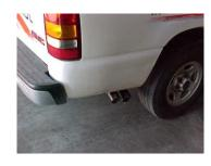
Install the stainless tips. Clamp down. To clean your stainless tips use any stainless cleaner or a Scotch Brite pad. Now go back and tighten all clamps, nuts and bolts. Start from the front and work back.
