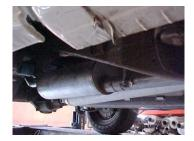
Install the driver side over axle tailpipe # D into the muffler. Use clamp # F to secure tailpipe to muffler. Do not tighten. Insert hanger into rubber grommet.
