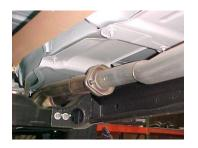
Lay out the exhaust on the floor so it looks like the drawing and compare parts with manual. To remove the stock exhaust un-bolt it from the 2-bolt flange located behind your factory Y-pipe. You will re-use your factory hardware. Leave all rubber grommets in place. Use WD-40 to aid in removal of exhaust and the
