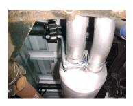
Install muffler #C onto head pipe 1-1/2" to 2" with the louvers facing towards the converter. Use a jack stand to support the muffler. Use clamp #G to secure the muffler to the head pipe. Do not tighten.
