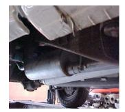
Install the driver side over axle tailpipe # D into the muffler. Use clamp # F to secure tailpipe to muffler. Do not tighten. Insert hanger into rubber grommet.
