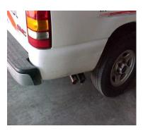
Install the stainless tips. Clamp down. To clean your stainless tips use any stainless cleaner. Now go back and tighten all clamps, nuts and bolts. Start from the front and work back.
