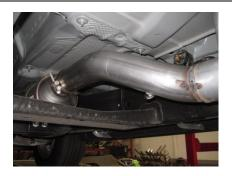
2.Install headpipe #A onto your factory pipe using your stock clamp insert welded hanger into the rubber grommet leave clamp loose.
