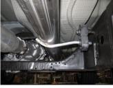
Next, install headpipe #A into the factory pipe. Insert welded grommet. Use factory clamp to secure, do not tighten.
