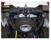
8. Install exit pipes #E. Use clamps #H to secure tailpipes. Do not tighten.
