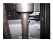
4. Slide muffler #B over headpipe 1.5-2" with the louvers facing towards the converter. Use a jack stand to support the muffler. Use clamp #E to secure the muffler to the headpipe. Do not tighten. Muffler inlet is looking into the louvers.
