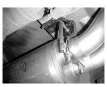
Install rear muffler hanger #H. Onto driver side outlet of the muffler, insert hanger into rubber grommet.
