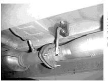
Install your head-pipe # A onto your existing stock flange, use your supplied hardware #J & K in the kit. Use a jack stand to support the converter. Insert the welded hanger into the rubber grommet.
