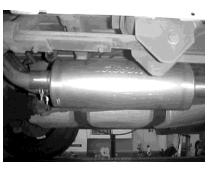
Install muffler #B onto head-pipe #A 1-1/2" to 2" with the louvers in the muffler facing towards the converter. Use a jack stand to support the muffler. Use Clamp #F to secure the muffler to the head-pipe. **Do Not Tighten at this Time!**
