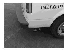
Install your Stainless Steel tips and clamp down. When you have everything in place \*, firmly tighten all your hardware and clamps securely down. To clean your stainless steel tips, use a stainless cleaner and polish.
