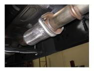
2. To remove your stock exhaust, unbolt the 2-bolt flange located in front of the muffler. Then cut off your tailpipe. Leave all rubber grommets in place.
