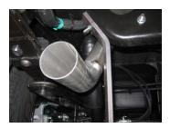
7. Install Spare tire Bracket on drivers side of Spare tire subframe as shown in the photo. Spare tire bracket will help keep the spare tire from rubbing on tailpipe. You will remove your factory spare tire heat shield. Be sure you have 1.5" clearance on all pipes near spare tire.
