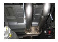
4. Install muffler #B onto headpipe #A 1.5-2" with louvers facing towards the converter. Use a jack stand to support the muffler. Use clamp #G to secure together. Do not tighten.
