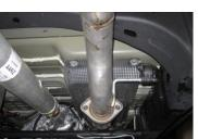
3. Install headpipe #A onto your existing stock 2-bolt flange. Use your factory nuts. Insert hanger into rubber grommet. Do not tighten. On short beds cut 12.5" headpipe
