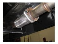
2. To remove your stock exhaust, unbolt the 2-bolt flange located in front of the muffler. Then cut off your tailpipe. Leave all rubber grommets in place. Use WD-40 to aid in the removal of the hangers from the rubber grommets.
