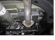
7. Install passenger side tailpipe #D into muffler 1.5-2". Insert welded hanger into rubber grommet. Use clamp #H to secure. Do not tighten. Install exit pipes #E onto tailpipes. Use clamps #H to secure pipes together. Do not tighten. Use zip ties to secure brake and fuel lines away from exhaust.
