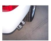
**8.** Install stainless steel tips #G. Clamp down. When you have everything in place, firmly tighten all bolts and clamps down securely. Use stainless steel cleaner and a Scotch Brite pad weekly to prevent tip from discoloration.
