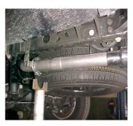
NEXT, INSTALL THE EXIT PIPES #E AND #F USEING CLAMPS #H TO SECURE TO THE TAILPIPES. DO NOT TIGHTEN.
