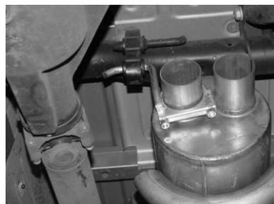
INSTALL MUFFLER #B ONTO HEADPIPE AT LEAST 1 1/2" TO 2". USE CLAMP #F TO SECURE MUFFLER TO HEADPIPE. DO NOT TIGHTEN. USE A JACK STAND TO SUPPORT THE MUFFLER. OUTLETS SHOULD BE AT THE TOP. INSTALL HANGER #I ONTO DRIVERSIDE MUFFLER OUTLET AND INSERT WELDED HANGER INTO GROMMET. DO NOT TIGHTEN.
