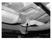
UNBOLT STOCK HEADPIPE AT THE 3 BOLT FLANGE DIRECTLY BEHIND THE CATALYTIC CONVERTER.
