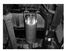
INSTALL MUFFLER #B ONTO HEADPIPE 1-1/2" TO 2" USING CLAMP #J. INSERT WELDED HANGERS INTO RUBBER GROMMET. MAKE SURE OUTLETS ARE LEVEL. USE A JACKSTAND TO SUPPORT MUFFLER. DO NOT TIGHTEN.
