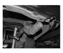
INSTALL EXIT PIPES # H ONTO OVERAXLE TAILPIPES USING CLAMP # I. ADJUST FOR YOUR PREFERENCE. NEXT ROTATE PIPES FOR BEST CLEARANCE AND ALIGN TO FRAME RAIL. TIGHTEN ALL CLAMPS AND BOLTS STARTING FROM THE HEADPIPE AND WORK BACK. INSTALL STAINLESS STEEL TIPS.
