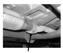
UNBOLT STOCK HEADPIPE AT THE 3 BOLT FLANGE DIRECTLY BEHINDTHE CATALYTIC CONVERTER. CUT STOCK TAILPIPE OFF RIGHT BEHIND THE STOCK MUFFLER. LEAVE ALL FACTORY RUBBER GROMMETS IN PLACE. SPRAY WD-40 ON ALL RUBBER GROMMETS FOR EASY REMOVAL.
