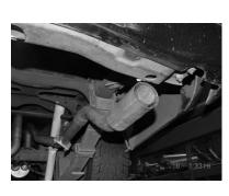
INSTALL EXIT PIPES # F ONTO OVERAXLE TAILPIPES USING CLAMP # J. ADJUST FOR YOUR PREFERENCE. NEXT ROTATE PIPES FOR BEST CLEARANCE AND ALIGN TO FRAME RAIL. TIGHTEN ALL CLAMPS AND BOLTS STARTING FROM THE HEADPIPE AND WORK BACK. INSTALL STAINLESS STEEL TIPS.
