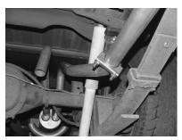
INSTALL PASSENGER SIDE TAILPIPE # C INTO THE MUFFLER 1-1/2" TO 2". ATTACH IT TO THE MUFFLER USING CLAMP # J USE CLAMP # J TO HOLD TAILPIPE TO HANGER # G. DO NOT TIGHTEN
