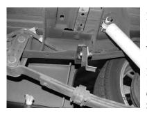
INSTALL HANGER # G ON THE PASSENGER TAILPIPE AND HANGER # H ON DRIVERSIDE TAILPIPE. MEASURE 19" FROM REAR OF FRAME AND BOLT INTO THE EXISTING ROUND HOLES (ABOUT 7/8") LOCATED ON THE FRAME ON BOTH SIDES OF THE VEHICLE.
