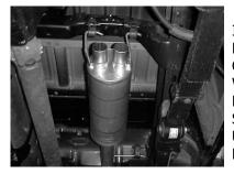
INSTALL MUFFLER #B ONTO HEADPIPE 1-1/2" TO 2" USING CLAMP #I + #k. INSERT WELDED HANGERS INTO RUBBER GROMMET. MAKE SURE OUTLETS ARE LEVEL. USE A JACKSTAND TO SUPPORT MUFFLER. DO NOT TIGHTEN.
