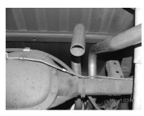
INSTALL DRIVERS SIDE FRONT TAILPIPE # D INTO MUFFLER 1-1/2" TO 2". USE CLAMP # I AND ATTACH IT TO THE MUFFLER. DO NOT TIGHTEN.
