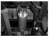
INSTALL MUFFLER #B ONTO HEADPIPE 1-1/2" TO 2" USING CLAMP #J. INSERT WELDED HANGERS INTO RUBBER GROMMET. MAKE SURE OUTLETS ARE LEVEL. USE A JACKSTAND TO SUPPORT MUFFLER. ATTACH HEADPIPE HANGER #K.
