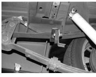
INSTALL HANGER # F ON THE PASSENGER TAILPIPE AND HANGER # G ON DRIVERSIDE TAILPIPE. MEASURE 19" FROM REAR OF FRAME AND BOLT INTO THE EXISTING ROUND HOLES (ABOUT 7/8") LOCATED ON THE FRAME ON BOTH SIDES OF THE VEHICLE.
