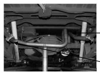
DO NOT TIGHTEN. INSTALL DRIVERS SIDE OVERAXLE PIPE # E ONTO FRONT TAILPIPE USING 'CLAMP #I. USE CLAMP # I TO HOLD TAILPIPE UP TO REAR HANGER # G.
