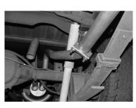
INSTALL PASSENGER SIDE TAILPIPE # C INTO THE MUFFLER 1-1/2" TO 2". ATTACH IT TO THE MUFFLER USING CLAMP # I. INSERT WELDED HANGER INTO RUBBER GROMMET AND USE CLAMP # I TO HOLD TAILPIPE TO HANGER # F. DO NOT TIGHTEN
