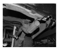
INSTALL EXIT PIPES # H ONTO OVERAXLE TAILPIPES USING CLAMP # I. ADJUST FOR YOUR PREFERENCE. NEXT ROTATE PIPES FOR BEST CLEARANCE AND ALIGN TO FRAME RAIL. TIGHTEN ALL CLAMPS AND BOLTS STARTING FROM THE HEADPIPE AND WORK BACK. USE ZIP TIES FOR BRAKE LINES AND ANY OTHER HOSES. INSTALL STAINLESS TIPS.
