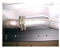
LAY OUT THE GIBSON EXHAUST ON THE FLOOR SO IT LOOKS LIKE THE DRAWING AND COMPARE PART #'S WITH MANUAL. TO REMOVE YOUR STOCK EXHAUST, REMOVE IT FROM THE STOCK 2-**BOLT FLANGE LOCATED** JUST BEHIND THE CONVERTER, LEAVING ALL RUBBER GROMMETS IN PLACE, USE WD-40 TO AID YOU IN REMOVAL OF EXHAUST AND HANGERS. DO NOT THROW AWAY **FACTORY** HARDWARE, YOU WILL RE-USE IT.
