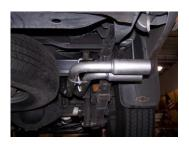
7. Install passenger side tailpipe #D into muffler 1.5-2" and attach with clamp #H. Use bolt kit #I to attach the tailpipes together. Do not tighten. Insert welded hanger into rubber grommet.
