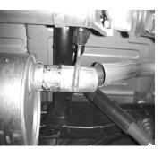
FOR EASIER REMOVAL OF THE STOCK EXHAUST CUT THE TAIL PIPE BEHIND YOUR MUFFLER. LUBE ALL RUBBER GROMMETS WITH WD-40. LEAVE ALL YOUR STOCK RUBBER GROMMETS IN PLACE.
