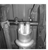
**INSTALL MUFFLER # B WITH** INLET TOWARDS Y-PIPE, WITH THE OUTLETS POSITIONED AT THE TOP OF THE MUFFLER. USE A JACK STAND TO SUPPORT THE MUFFLER. USE CLAMP #F TO CONNECT THE MUFFLER TO HEADPIPE. INSTALL HANGER # H ONTO THE DRIVERSIDE OUTLET OF THE MUFFLER. INSERT THE WELDED HANGER INTO THE RUBBER GROMMET FROM THE PASSENGER SIDE. DO NOT TIGHTEN.
