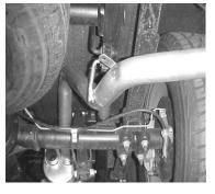
MAKE SURE MUFFLER OUTLETS ARE LEVEL **BEFORE INSTALLING** TAILPIPES. NOW INSTALL PASSENGER TAILPIPE #C. INSERT WELED HANGER INTO RUBBER GROMMET.
