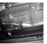
LAY OUT THE GIBSON EXHAUST ON THE FLOOR SO IT LOOKS LIKE THE DRAWING. AND COMPARE PARTS WITH MANUAL. UN-BOLT THE STOCK FLANGE BEHIND FACTORY Y-PIPE. KEEP THE STOCK **BOLTS, NUTS** FOR YOU WILL RE-USE THEM.
