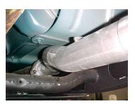
Lay out the exhaust on the floor so it looks like the drawing and compare parts with manual. To remove the stock exhaust, remove it from the stock 2-bolt flange located just behind the catalytic converter. Leave all rubber grommets in place. Use WD-40 to aid in removal of exhaust and the hangers. Do not discard your factory hardware. You will re-use it.
