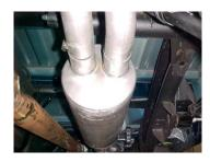
Install muffler onto head pipe #A 1-1/2" to 2" with the louvers facing towards the converter. Use a jack stand to support the muffler. Use clamp #H to secure the muffler to the head pipe. Do not tighten. Muffler inlet is looking into the louvers. The muffler outlets should be at the top.
