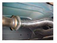
Install head pipe # A onto you're existing stock 2-bolt flange. Re-use your stock hardware to secure. Insert welded hanger into rubber grommet. Use a jack stand to support the converter. Do not tighten.
