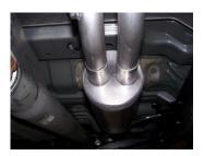
4. Install muffler (**#B**) onto headpipe (**#A**) 1.5-2" with louvers facing towards the converter. Use a jack stand to support the muffler. Outlet of muffler will be level.
