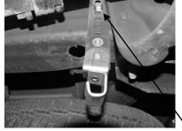
INSTALL METAL HANGERS (#H) INTO HOLES LOCATED APPROX. 16" FROM THE REAR OF THE FRAME. METAL HANGERS ARE MOUNTED ON THE OUTSIDE OF FRAME. USE THE HARDWARE PROVIDED. THE BOLT AND WASHER WILL GO INTO THE 3<sup>RD</sup> HOLE FROM THE TOP OF THE HANGER. YOU MAY NEED TO LOOSEN SPARE TIRE FOR EASIER REMOVAL.
