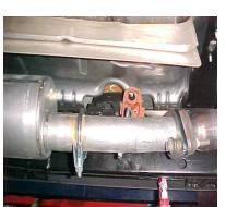
INSTALL HEADPIPE #A. SLIDE HEADPIPE INTO MUFFLER 1-1/2" TO 2" USE CLAMP # F TO SECURE HEADPIPE TO MUFFLER. DO NOT TIGHTEN. NEXT USE YOUR STOCK NUTS AND BOLTS TO SECURE HEADPIPE TO STOCK FLANGE.
