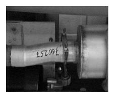
SLIP HEADPIPE #A ONTO THE STOCK EXTENSION PIPE BEHIND THE CONVERTER. ALIGN NOTCH WITH STOCK HEADPIPE PIN.SLIP MUFFLER WITH THE LOUVERS INSIDE OF THE MUFFLER FACING FORWARD ONTO HEADPIPE #A NO LESS THEN 1-1/2" AND NO MORE THEN 2". THEN INSTALL FRONT MUFFLER HANGER #G AND REAR MUFFLER HANGER # H. DO NOT TIGHTEN. USE A JACKSTAND TO SUPPORT THE MUFFLER, MUFFLER INLET IS LOOKING INTO THE LOUVERS.
