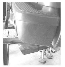
INSTALL THE STAINLESS TIP. USE ANY ALUMINUM OR STAINLESS STEEL CLEANER TO POLISH YOUR STAINLESS STEEL TIP. NOW GO BACK AND TIGHTEN THE FLANGE AT THE CATALYTIC CONVERTER, HANGER AND CLAMPS.
