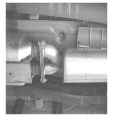
INSTALL MUFFLER ASSEMBLY ONTO THE STOCK FLANGE REUSING THE FACTORY GASKET AND HEADPIPE BOLT KIT #E. DO NOT TIGHTEN!!
