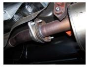
**2.** Remove the 2-bolt flange in front of your stock muffler. Also remove exit pipe from the clamp at the rear. Leave all rubber grommets in place. Use WD-40 to aid in removal of exhaust and hangers.
