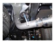
7. Install the exit pipe #D on the tailpipe. Secure together with clamp #E. Do not tighten. Roll the exit pipe until it is at the correct angle for your truck. Insert the welded hanger into rubber grommet.
