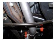
**6.** Install the over axle tailpipe #C into the extension pipe 1½-2". Use clamp #E to secure. Do not tighten. Insert welded hanger into the rubber grommet.
