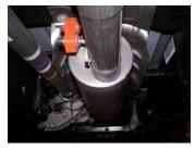
**5.** Install muffler #B onto headpipe 1½"-2" with the louvers facing towards the converter. Outlet will be at the 6 o'clock position. Use a jack stand to support the muffler. Use clamp #E to secure the muffler to the headpipe. Do not tighten. Muffler inlet is looking into the louvers.
